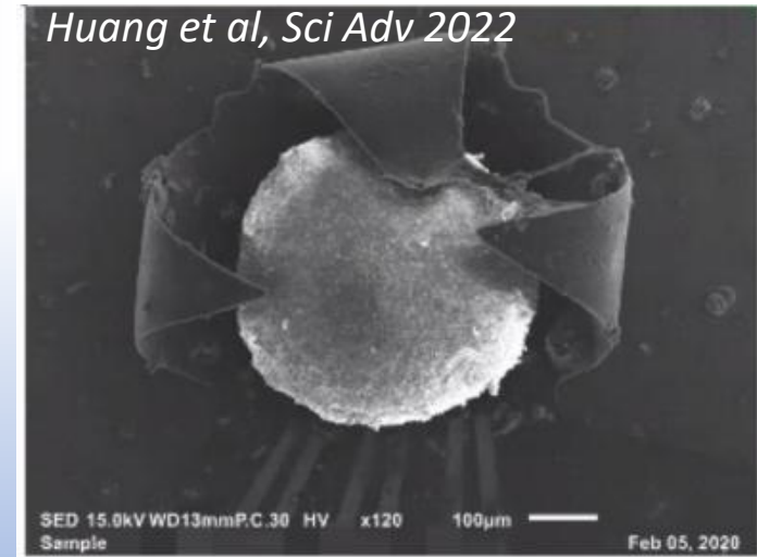
Human brain organoid caged in shell electrodes
