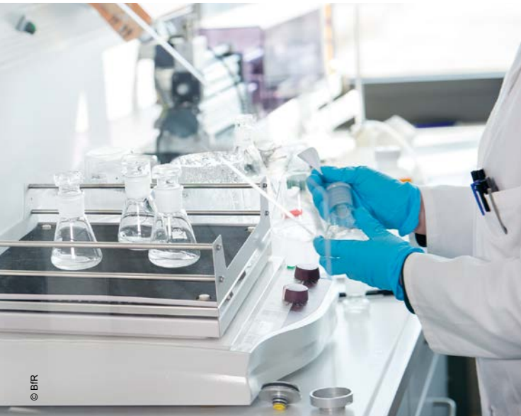
Shaken and checked: the vapour's components are extracted from the smoking machine's filter pad and then analysed.
