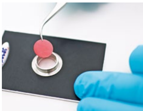
For analysis using Fourier transform infrared spectrometry, a pellet is made from the inks to be tested and then analysed.
