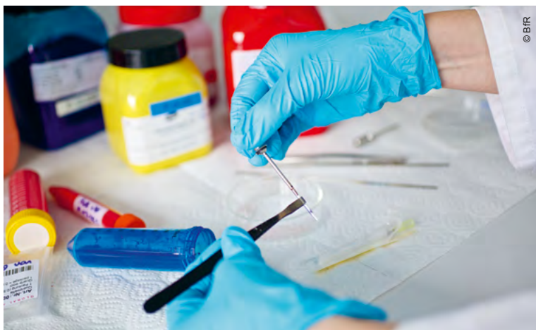
Colour pigments are filled into test tubes for thermal treatment by means of pyrolysis.
